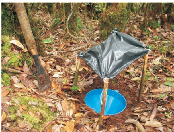
Figure 1. A pitfall trap showing the funnel, plastic sheet and four wooden sticks. A bottle containing alcohol was placed under the funnel. Note the hole cutter (candak) that was used to dig the pitfall trap.
